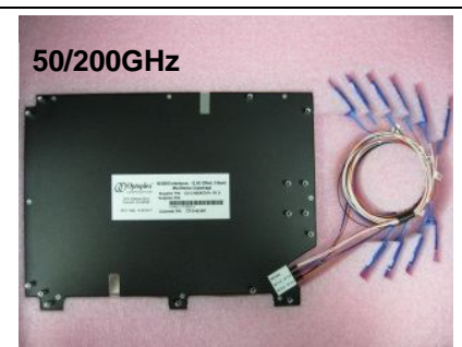
Figure 33 - 50/200GHz Two-Stage Mux/DeMux Co-Packaged Interleaver Module.
