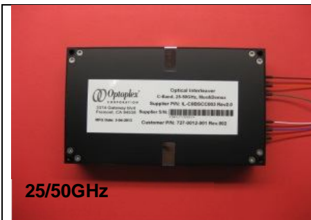
Figure 31 - 25/50GHz Mux/DeMux Co-Packaged Interleaver Module.
